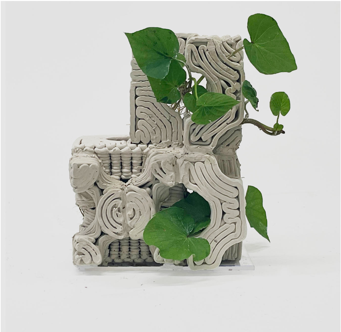
Figure 6. An early mockup assembling featuring twelve peices of ceramic printed geometry in stoneware , for the habitat of the woodrat.
